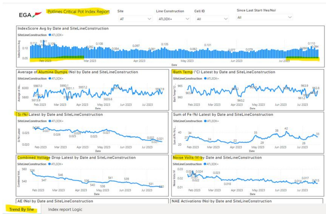
Figure 6. Trend by line page – index score and KPI analysis of the potline.
